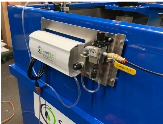
Ozone Generator on SmartSkim Coolant Recycling System
