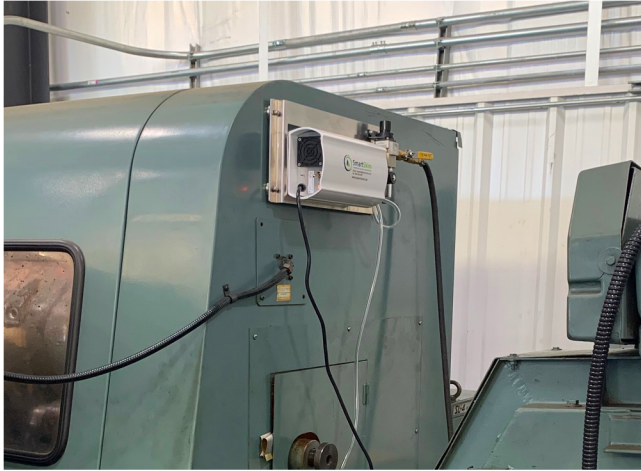
Ozone Generator retrofitted to CNC Machine
